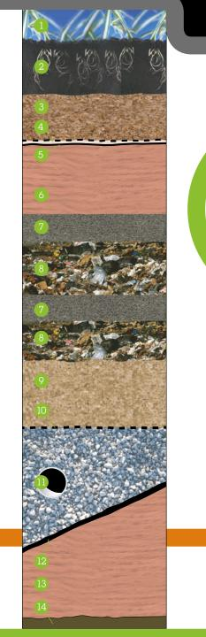
This illustration depicts a cross section of the standard environmental protection technologies of modern landfills. While the technologies used in most landfills are similar, the exact sequence and type of materials may differ from site to site depending on design, location, climate and underlying geology.
